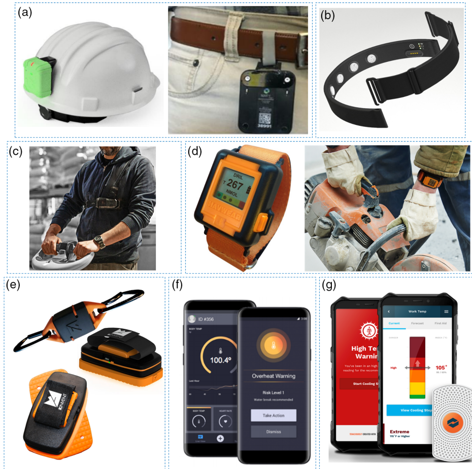
Figure 2. Examples of wearables for occupational safety monitoring. a) The Triax Proximity Trace consists of TraceTags affixed to hard hats for monitoring safe working distance and interactions. b) The SmartCap LifeBand measures brain waves to estimate alertness and fatigue levels at work. c) The StrongArm ErgoSkeleton Lift Assist helps with heavy lifting by transferring the load from the upper body and back to the legs. d) Reactec HAVwear is designed for the risk management of hand arm vibrations and provides real-time safety analytics and alerts. e) K-invent dynamometers consist of force transducers with biofeedback to evaluate muscle strength and endurance. f) Kenzen's personalized app and smart PPE enable the continuous safety monitoring of workers by tracking the microclimate, core body temperature, heart rate and exertion. g) The Corvex Temperature Management platform monitors the work temperature of frontline workers, providing them with situational awareness and data transparency. The figures were reproduced with permission: a) Reproduced with permission. [61] Copyright 2021, Triax; b) Reproduced with permission. [118] Copyright 2021, SmartCap; c) Reproduced with permission. [45] Copyright 2021, StrongArm; d) Reproduced with permission. [62] Copyright 2021, Reactec; e) Reproduced with permission. [139] Copyright 2021, K-invent; f ) Reproduced with permission. [82] Copyright 2021, Kenzen; and g) Reproduced with permission. [230] Copyright 2021, Corvex.
